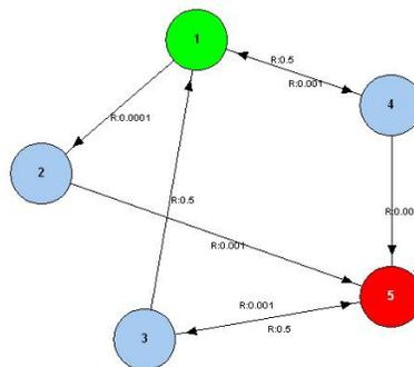
**FIGURE 7 A MARKOV MODEL USED FOR CALCULATING THE LIKELIHOOD OF A STATE CHANGE**
