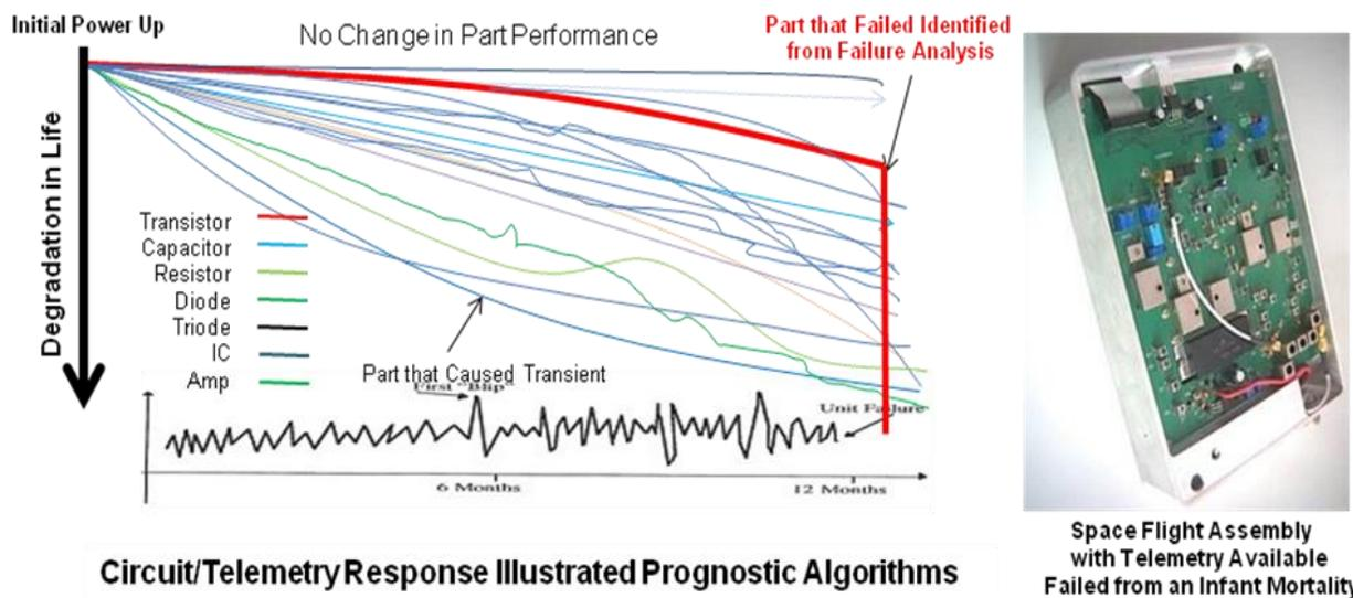
**FIGURE 8 CIRCUIT/ASSEMBLY TRANSIENT BEHAVIOR OCCURRS AS PARTS AGE PREMATURELY IS THE REASON PREDICTIVE ALGORITHMS CAN MEASURE EQUIPMENT USABLE LIFE USING ANALOG TELEMETRY**
