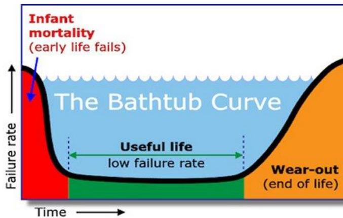
**FIGURE 6 RELIABILITY ANALYSIS ENGINEERING’S BATHTUB CURVE**
