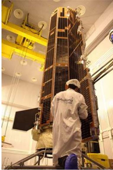
**Figure 11. The ESA GOCE Satellite/Gradiometer during Factory Integration & Test**
