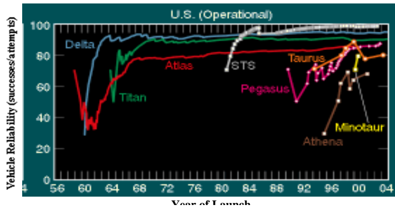
FIGURE 1 FORTY-EIGHT YEARS OF RELIABILITY OF U.S. LAUNCH VEHICLES USING TESTING TO INCREASE RELIABILITY (AEROSPACE CORPORATION)
