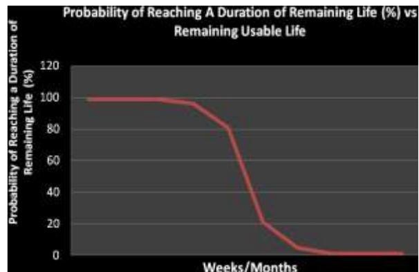
Figure 11 Proprietary Cumulative Distribution used to Determine Spacecraft Equipment Remaining-Usable-Life in a Non-Markov Paradigm
