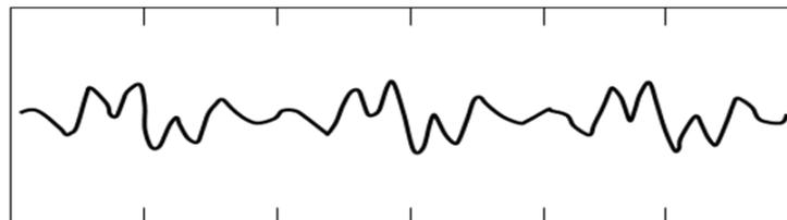
**FIGURE 6 TIME DOMAIN LOW FREQUENCY STEADY-STATE INFORMATION SIGNAL WITH PHASE MODULATION**
