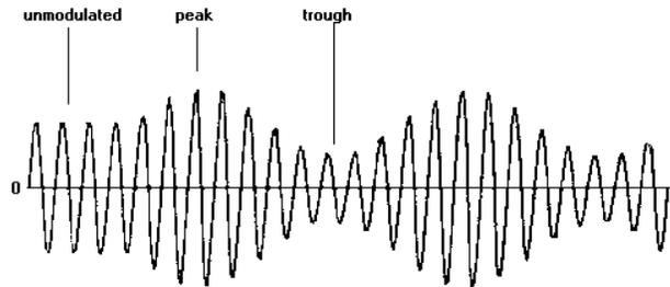
**FIGURE 4 AMPLITUDE UNMODULATED PORTION AND MODULATED SIGNAL**
