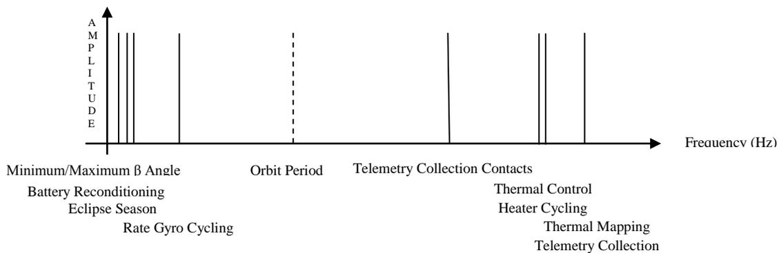
**FIGURE 11 FREQUENCY SPECTRUM (POSITIVE FREQUENCIES) FOR BOEING GPS BLOCK I SATELLITE**
