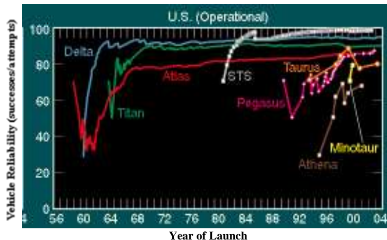
Figure 2. The Achieved Reliability of U.S. ICBMs and Launch Vehicles not Employing Intelligent, Self-Prognostic Equipment from 1957 through 2004 (Aerospace Corporation, 2005).
