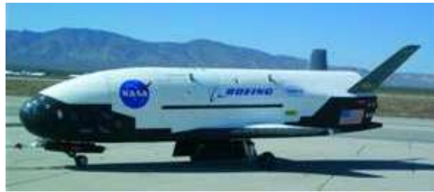
Figure 9. The Classified Boeing/NASA/Air Force 30 ft. X-37, Human Rated Reusable Spacecraft without Intelligent, Self-Prognostic Equipment, Launched to Obtain Long-Duration, Automated Space Flight Data, Reentry Flight Characteristic Data and Automated Payload Deployment Data.
