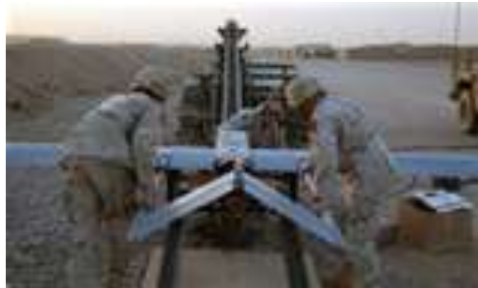
Figure 6. The Intelligent, Self-Prognostic, Reliability-Centered Army/Rockwell Collins Shadow UAV using Embedded Predictive Algorithms from its PHM Program to Measure On-Board Equipment Remaining Usable Life for Down-Linking in Real-Time to Shadow Maintenance Crew.
