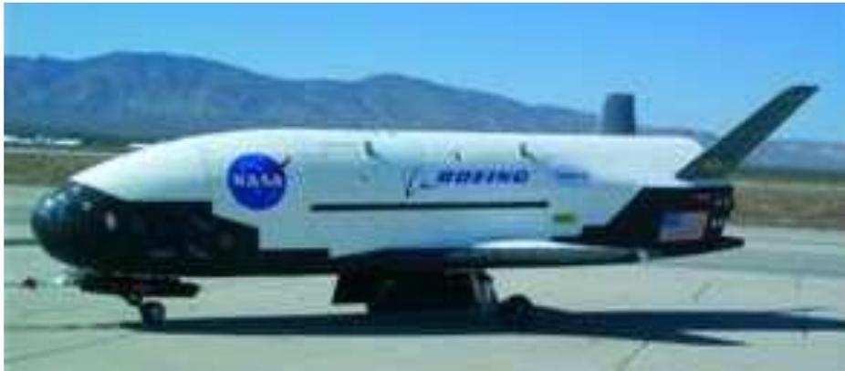
**Figure 10. The Classified Boeing/NASA/Air Force 30 ft. X-37, Human Rated Reusable Spacecraft without Intelligent, Self-Prognostic Equipment, Launched to Obtain Long-Duration, Automated Space Flight Data, Reentry Flight Characteristic Data and Automated Payload Deployment Data.**
