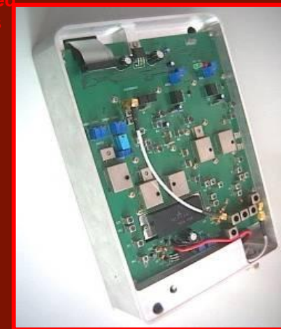
Space Flight Assembly with Telemetry Available Failed from an Infant Mortality 12
