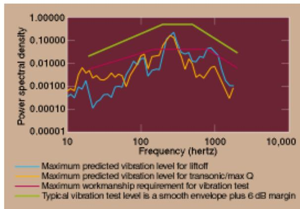
**Figure 6: Typical Vibration Energy Levels Used During Contractor Factory Acceptance Testing Specified In Contract (Aerospace Corporation <sup>13</sup>)**
