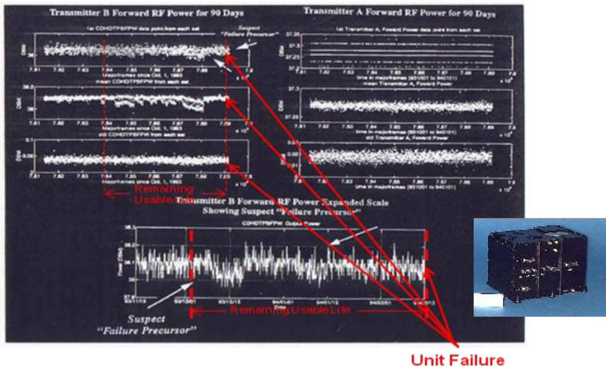
Figure 19. Results from Measuring Transmitter remaining Usable Life on the EUVE Satellite TDRSS RF Transmitter using the Forward RF Power Telemetry Transducer Output (Post Processing Results using Predictive algorithms).<sup>9</sup>
