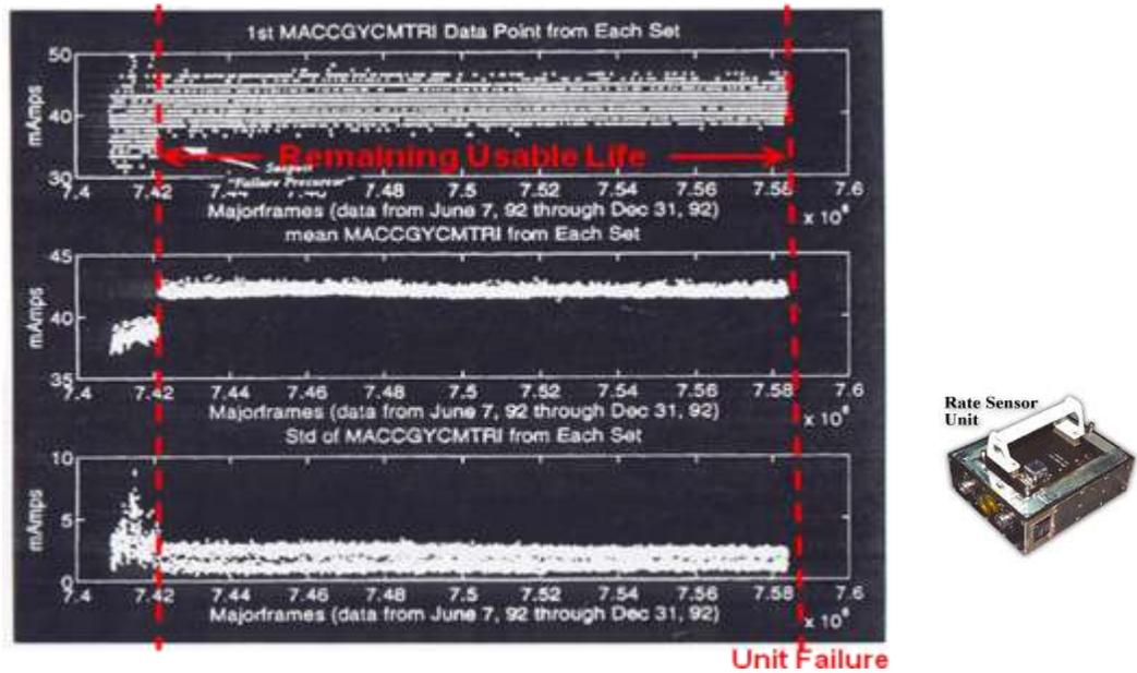
Figure 18. Results from Measuring Rate Gyro Remaining Usable Life using Rate Gyro Motor Current Telemetry Transducer Output (Post Processing Results).<sup>9</sup>
