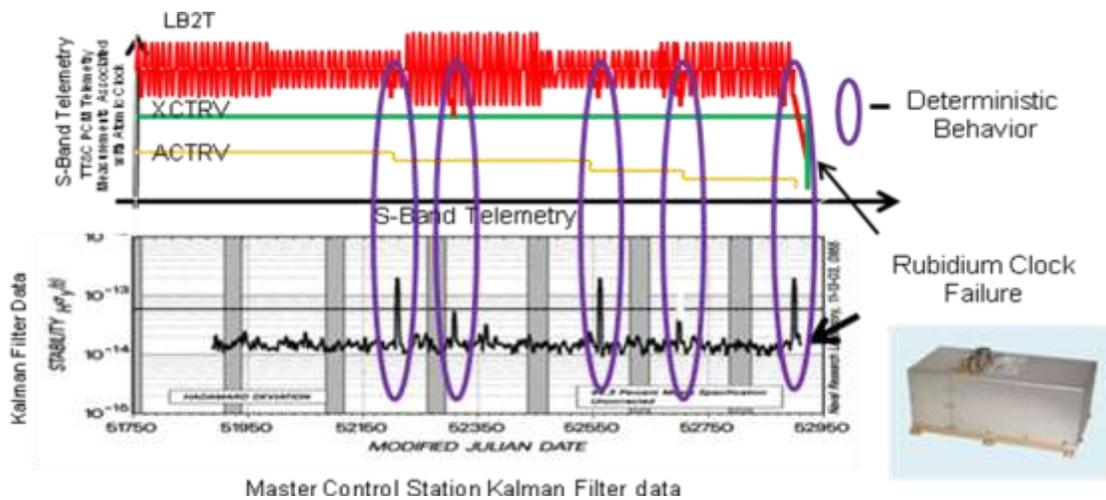
Figure 15. The Prognostic Analysis Completed on a GPS On-Orbit Satellite Rubidium Atomic Frequency Standard Illustrating Transient/Deterministic Behavior caused from Accelerated Aging (circa 1983).
