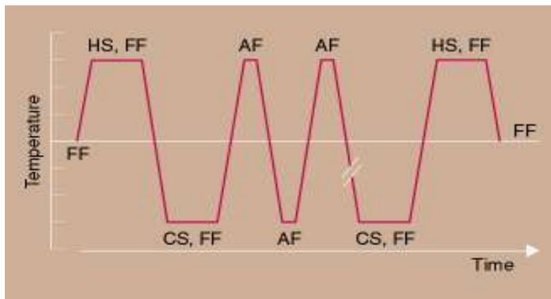
**Figure 9: Typical Thermal/Vacuum Profiles Used During Contractor Factory Acceptance Testing Specified In Contract (Aerospace Corporation <sup>13</sup>)**
