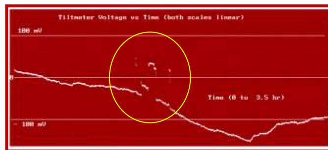
**Figure 4. Example of the Transient Behavior in Equipment Telemetry caused from Accelerated Aging that's often Present in Normal Appearing Data from Fully Functional Equipment, Misdiagnosed as Noise**
