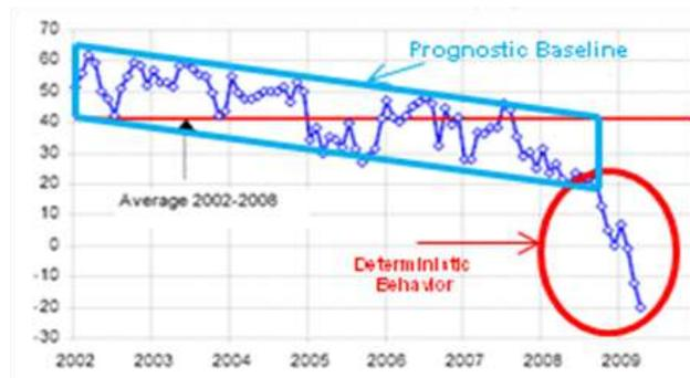
**Figure 13. Example of a Prognostic Analysis Illustrating Non-Repeatable Transient Behavior/Early Signs of Premature Aging//Prognostic Markers/Prognostic Identifiers in Equipment Telemetry Caused from Accelerated Aging.**
