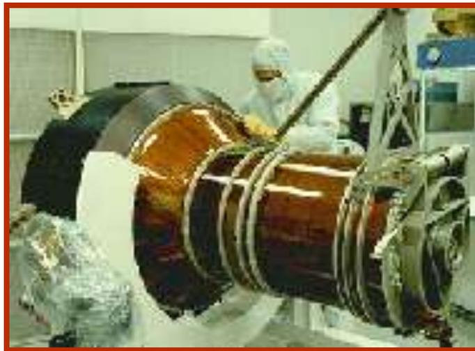
**Figure 17. NASA/U.C. Berkeley Extreme Ultra Violet Explorer Telescope Payload Designed and Built by U.C. Berkeley Space Sciences Laboratory to Function 10 Years On-Orbit and be Replaced by an Astronaut**
