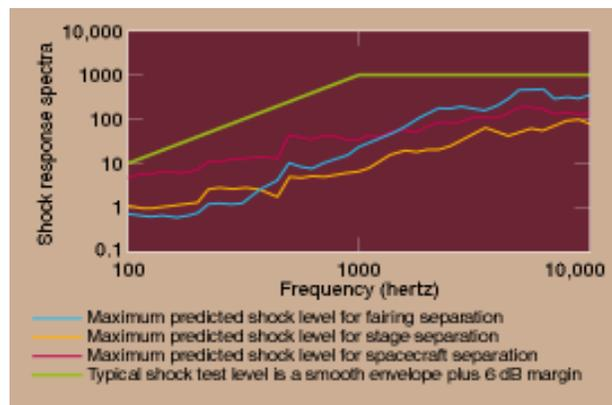
**Figure 8: Typical Shock Energy Levels Used During Contractor Factory Acceptance Testing Specified In Contract (Aerospace Corporation <sup>13</sup>)**
