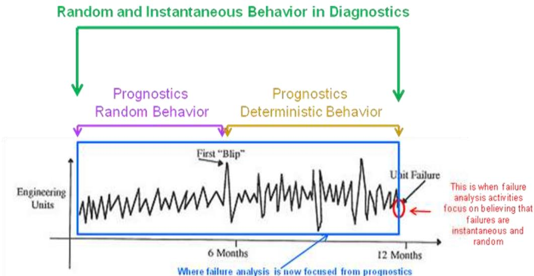
**Figure 12. Comparisons between Definitions of Duration between Equipment Beginning-of-Life and End-of-Life Based on Diagnostic Analysis and Prognostic Analysis.**
