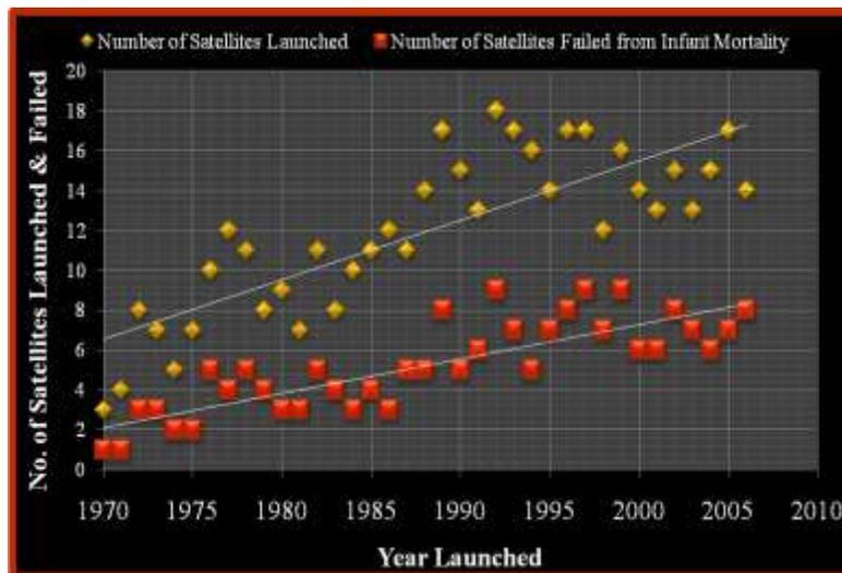
**Figure 3. Number of Civil and Commercial Satellites Launched per Year (Gold) and the Number that Failed Prematurely (Red). (Frost & Sullivan<sup>12</sup>).**
