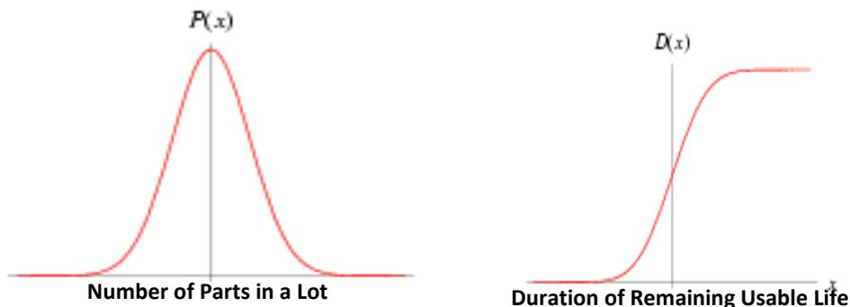
**Figure 10. Proprietary Piece-Part Probability Distribution Function Generated by Parts Suppliers that Defines the Likelihood of a Part Failing Prematurely and the Integral of the Piece-Part Normal Distribution**
