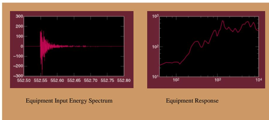
**Figure 7: Typical Shock Energy Input and Response Levels Behavior during Contractor Factory Acceptance Testing (Aerospace Corporation <sup>13</sup>)**
