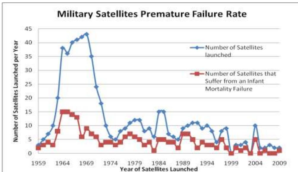
**Figure 2. The Number of (Unclassified) Military Satellites Launched and the Number of Unclassified Military Satellites that Failed Prematurely Starting from 1959 (Futron Corp. <sup>15</sup>).**
