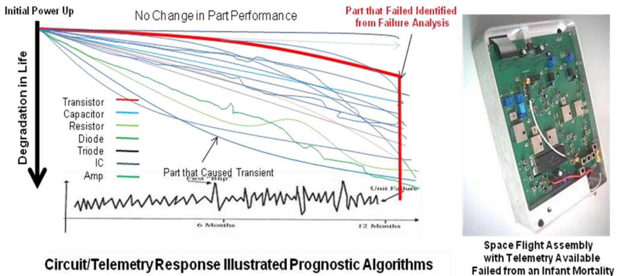
**Figure 10. The Reason Predictive Algorithms can Measure Equipment Usable Life using Equipment Telemetry by Illustrating Accelerated Aging caused from a Part that is Aging Prematurely in Performance**
