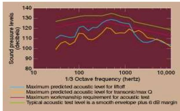
**Figure 5: Typical Acoustic Radiated Energy Levels Used During Contractor Spacecraft Factory Acceptance Testing Specified In Contract (Aerospace Corporation <sup>13</sup>)**
