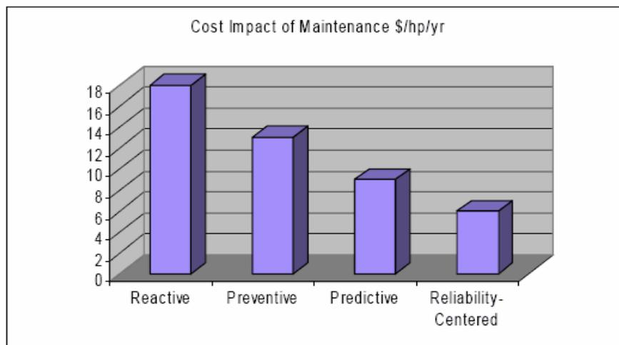
**FIGURE 5 THE RELATIVE COST OF DIFFERENT MAINTENANCE PROGRAMS.
