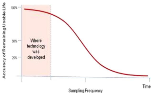
**Figure 9 Achieved Accuracy of Measured RUL vs. Sample Frequency Used in Analysis <sup>9</sup>**
