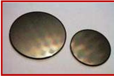
**Figure 21 EUVE Telescope Multi-Plate Channel (MPC) EUV Photon Detectors**
