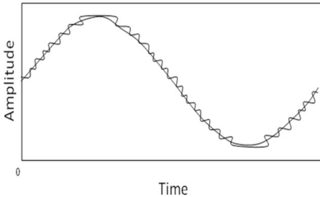
**Figure 4 A Diagram Illustrating that Digital Telemetry is Sampled Analog Data**
