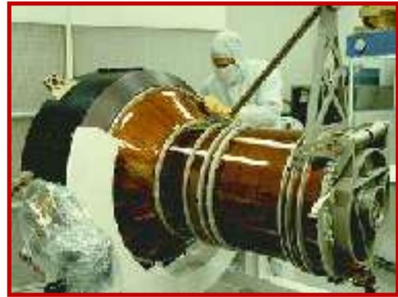
**Figure 18 NASA/U.C. Berkeley EUV Telescope during Assembly**
