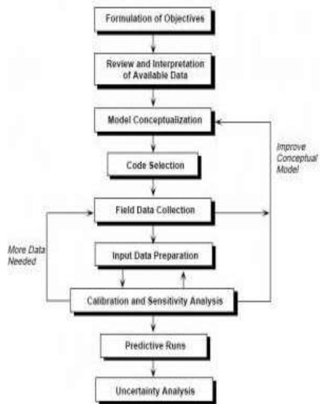
**Figure 3 A Process used to Develop a Proprietary Model-Based Predictive Algorithm.**
