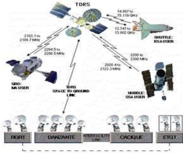
**Figure 16 The NASA Space-Based Telemetry System for Routing Spacecraft Telemetry to the SSL CEA**
