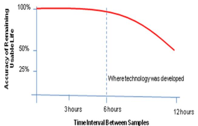
**Figure 11 Achieved Accuracy of the Measured Remaining Usable Life vs. Duration between Samples of Telemetry <sup>9</sup>**
