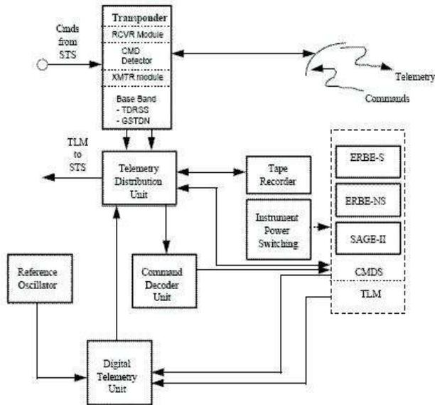
**Figure 20 NASA EUVE STDN/TDRSS C&DH Subsystem Block Diagram**
