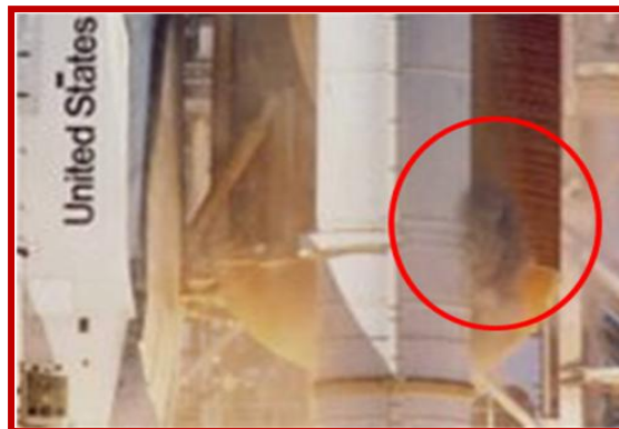
FIGURE 5 THE SPACE SHUTTLE CHALLENGER SRM O-RING FAILURE OF THE SPACE SHUTTLE CHALLENGER “O” RING WAS RECORDED ON VIDEO BEFORE LIFT-OFF ON THE LAUNCH PAD
