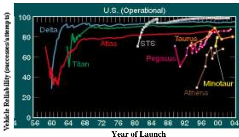
Figure 1. Forty-Eight Years of Reliability of U.S. Launch Vehicles using Testing to Increase Reliability (Aerospace Corporation)
