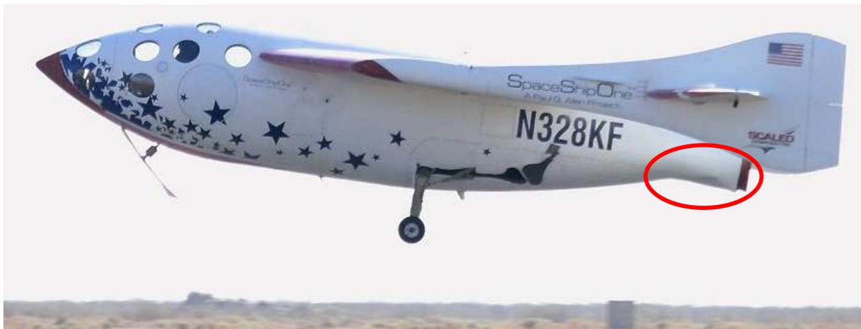
**Figure 1. The Damaged Virgin Galactic Commercial, Manned SpaceShip1 without Intelligent, Self-Prognostic Equipment Returning for Landing after Reaching Suborbital Altitude in 2009 Winning the \$10M Ansari X-Prize with Damage to the Bottom Rear Fuselage Clearly Visible from the Detachment of the Solid Rocket Motor during Suborbital Injection Preventable by using a PHM.<sup>17</sup>**
