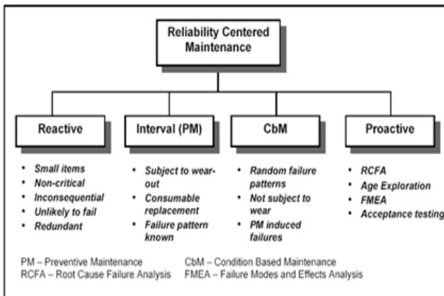
**Figure 6. Components of a Reliability Centered Maintenance Program.**
