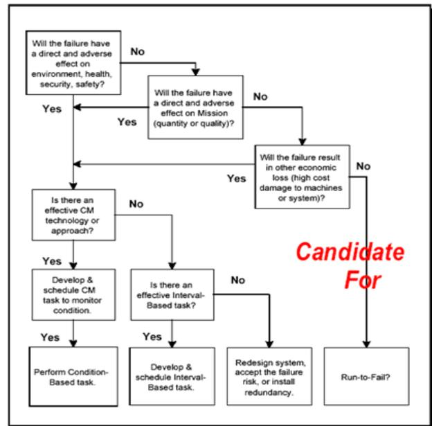
**Figure 7. An Example of a Reliability Centered Maintenance (RCM) Logic Tree.**
