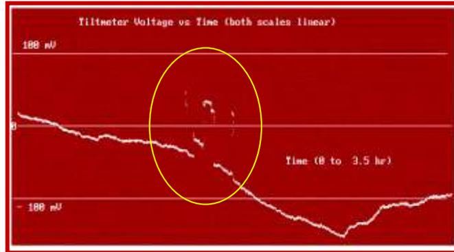
**FIGURE 1 EXAMPLE OF THE TRANSIENT BEHAVIOR IN EQUIPMENT TELEMETRY CAUSED FROM ACCELERATED AGING DIAGNOSED AS NOISE**
